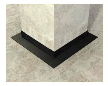
Cut another piece of the membrane enough to cover the entire corner angle. This must be done for all the corner joints. Then proceed with the application of the first layer of the bituminous membrane.
