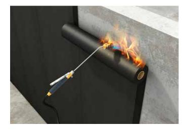
If a recess has not been provided for a membrane in a vertical wall, a nailed and sealed profile must be fitted as an end finish for the membrane bonded to the wall.
