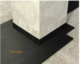
Apply again another piece of membrane on top of the fisrt layer, now on the opposite side of the corner. In this case, the overlapping should have an angle of 45°.
