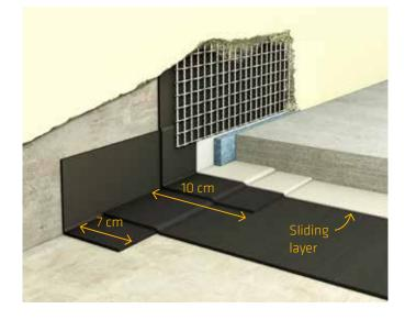
If the waterproofing membrane comes up to the top of perimeter walls, it must then be covered with a nailed flashing.
